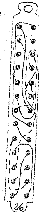
FIG. 4. SLIDE. SHOWING PRINTED CIRCUIT.
