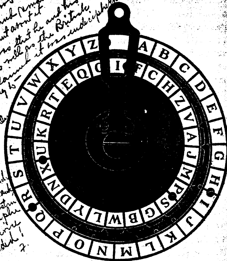
Plett's Cipher Machine, a modification of the famous Wheatstone cryptograph. The inner disk contains twenty-six spaces, the outer twenty-seven. The machine is so constructed that with each revolution of the inner disk it changes its position one space. The alphabet may be changed at will.
